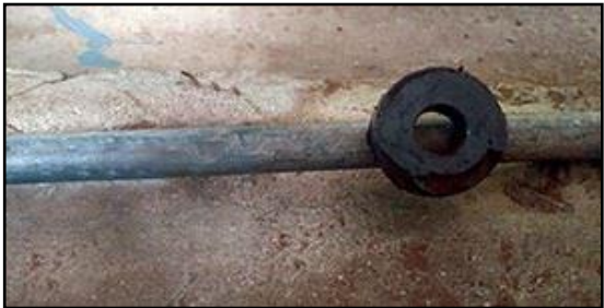
Galvanized Steel: The scratched area will remain a dull gray. A magnet will stick.
