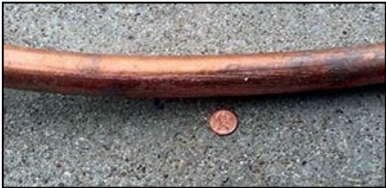
Copper: The pipe may appear dull brown on the outside but will be the color of a bright penny if gently scratched. A magnet won't stick.
